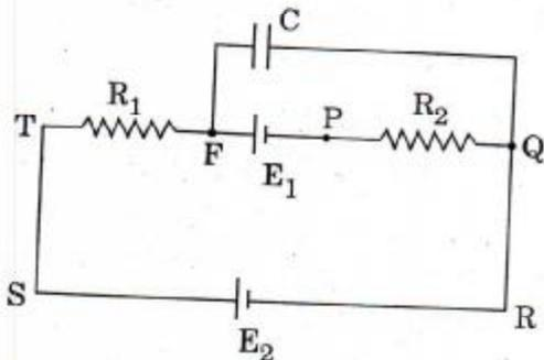
In the circuit given here,  $C = 2 \mu F$ ,  $R_1 = 3 \Omega$ ,  $R_2 = 5 \Omega$ ,  $E_1 = 12 V$ ,  $E_2 = 16 V$ .
